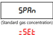
If you press the setting button once again while "SPAn" is displayed, the set calibration gas concentration is displayed as a number.
