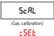
When the calibration gas concentration change is completed, it is displayed as "ScAL". In this state, if the setting button is pressed, the current concentration is displayed. (If the concentration is different from the value of the standard gas when the concentration is held after the standard gas is injected)
