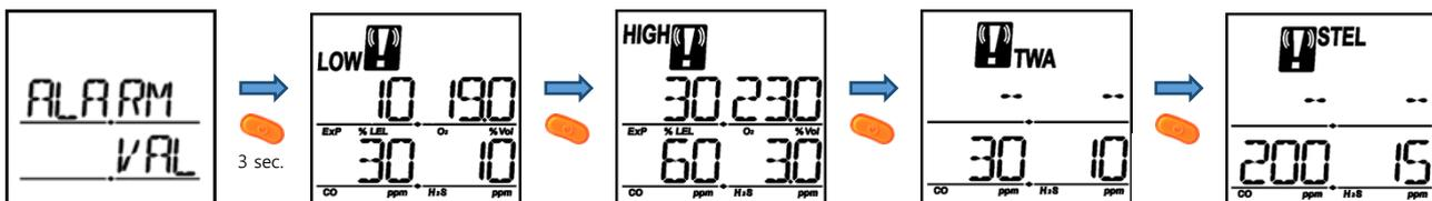
Press the KEY button (
