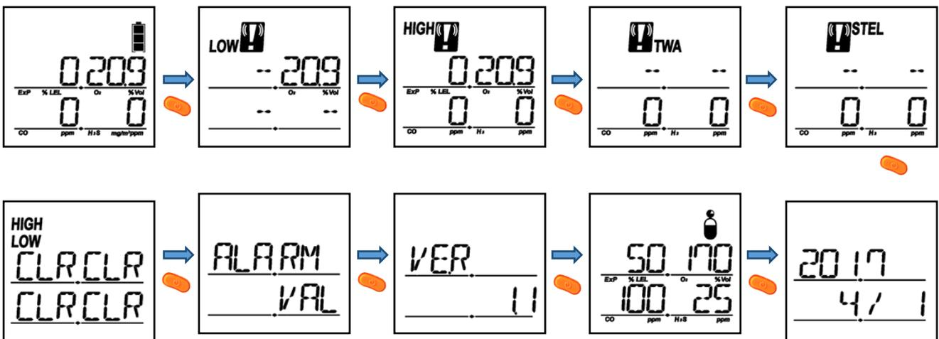
The displays in ten different modes as above are shown in the measuring mode every time when you press the KEY button(
