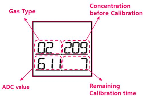
**Initial Standard gases concentration for calibration**
